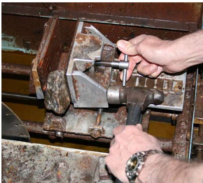
Figure 3. To secure the specimen in the vise, tap on the corner of the back jaw to release any binding that may be present.
