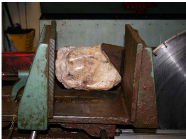
Figure 5. Notice the wood wedge to the right of the rock, helping to stabilize the specimen in the vise.
