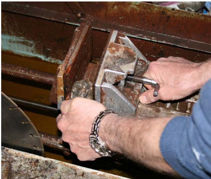
Figure 2. Grip the rock firmly to make sure that it will not move in the vise.
