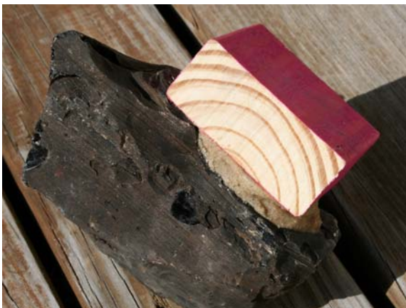
Figure 4. Medium-size piece of obsidian glued to a piece of 2 x 4, ready to be sawed. Notice the thick layer of sand and glue between the rock and the board.
