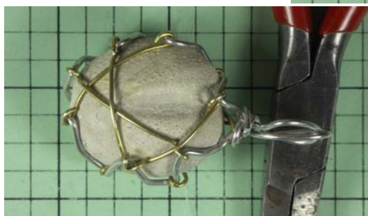
Figure 11 – Bend each end of the aluminum wire into a loop and then secure the ends around the base of the loop.
