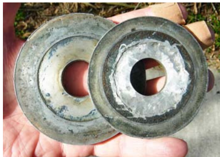
An overhanging rock milled one of these flanges before the blade was bent.
