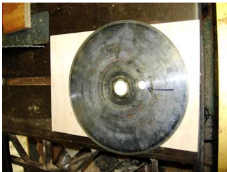
Flattening of the blade is done on a ¼-inch plywood surface.
