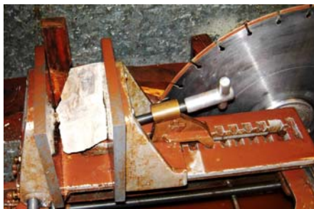
Use wedges when clamping irregular rocks
