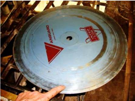
Test for flatness by using your finger to tap around the perimeter of the saw.
