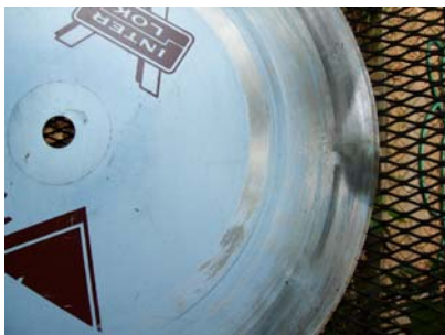
The saw only cut an inch before the glue joint broke.
