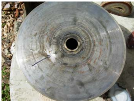
The arrow is pointing to a ½-inch wide and 1/8-inch deep dent.
