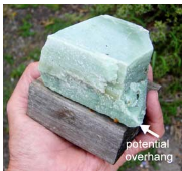
Rock glued to a board. The rock extends beyond the board on the right and is a potential overhang. Clamp it with the point on top.
