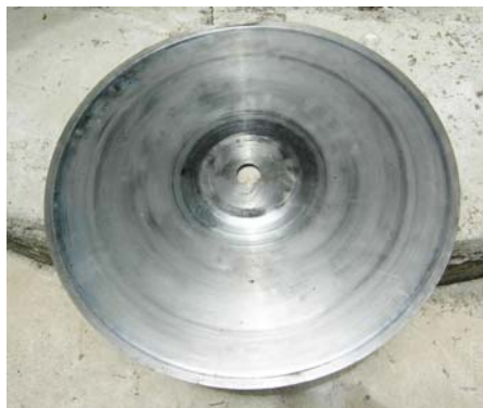
The rock hit the flange, rotated in the clamp, and dished the blade by 1/4 inch.
