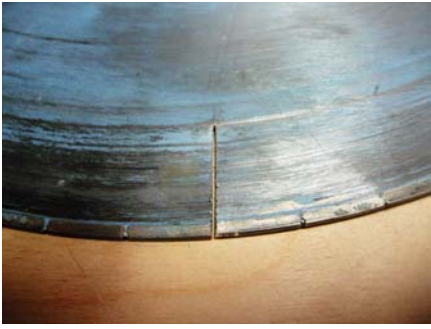
Gently hammer out the bend on the plywood.
