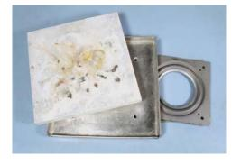
All you need to make one of these is a piece of aluminum sheet and an inexpensive turn table assembly. A good hardware store will have both, although you can usually find the aluminum in the scrap pile of a local sheet metal shop.
