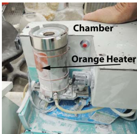
Rear view of the powder chamber of a Swam Blaster with the orange heater.
