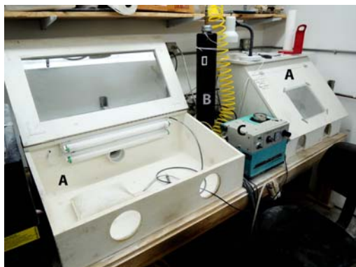
A: Blast cabinet. B: Silica Gel tower. C. Swam Blaster
