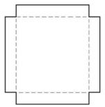
bend the sides along the dotted lines to form a tray that cradles the solder pad. I attached the tray to the turntable assembly with a couple small machine screws and nuts.
