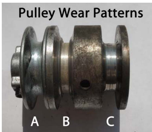
Pulley Wear Patterns: A: new , B: a step is worn into the pulley, C: belt has worn the slot square and polished the bottom.
