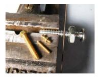
ping the bolt by the piece to be sawed off localizes any crushing damage to the piece that will be thrown away.
