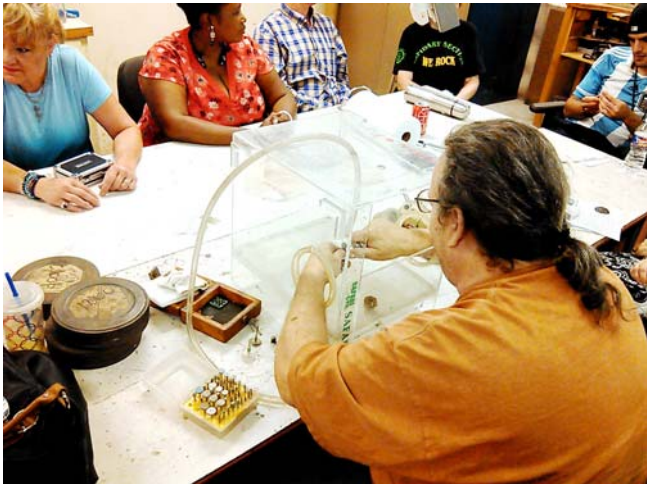
Edward Clay carving a cabochon. Water runs continuously on the stone to keep it cool.
