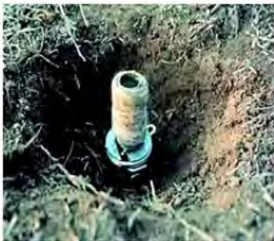
When the trap is set, only the capsule holder and capsule protrude above ground level.
