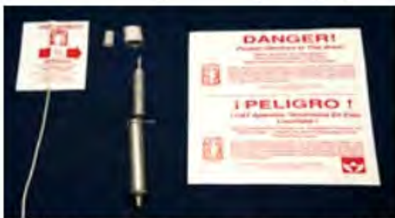
The M-44 consists of a capsule holder, a cyanide capsule, a spring-activated ejector, and a stake. Bilingual signs warn about the device.
