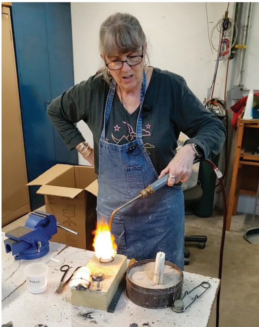
Casting using Cuttlefish Molds
