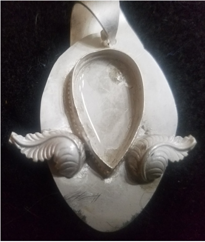
Top: The “Water Test” demonstrates the bezel is soldered correctly in place.
