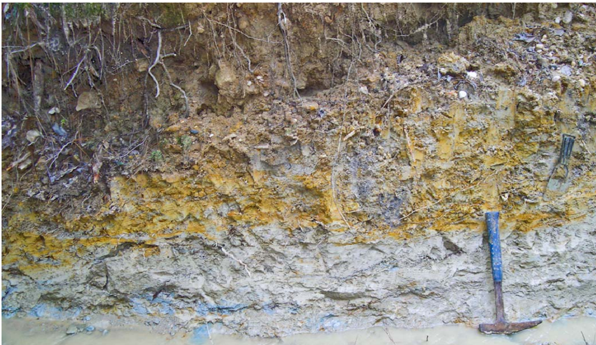
Figure 13. Catahoula Formation / Fleming Formation contact at the origin of both Transect 1 and Transect 2. Sample C1 and M1 were both taken from the area encompassed by this photo. Geologist pick handle is 13 in (33 cm) in length. Paint scraper is in the lower Fleming Formation.
