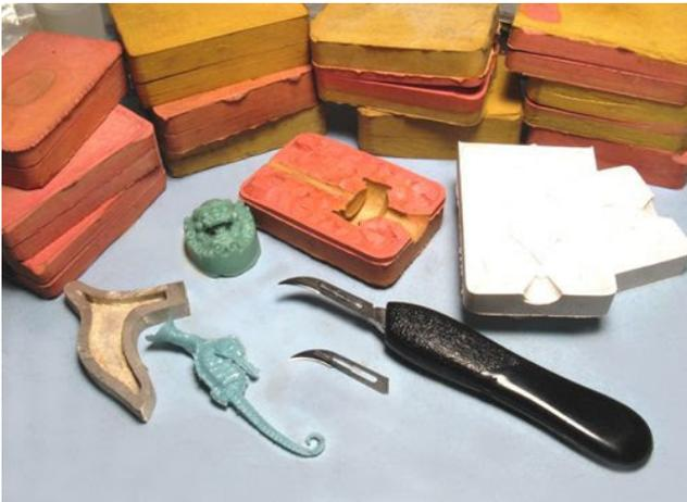
The #11 blade is triangle shaped, and the #12 is hawksbill shaped. I find the hawksbill is particularly nice for cutting the registration keys of the mold.
