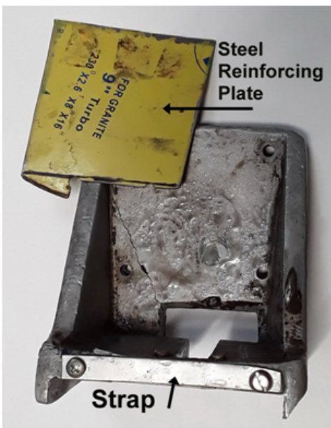
Fixing the rock clamp with a steel plate
