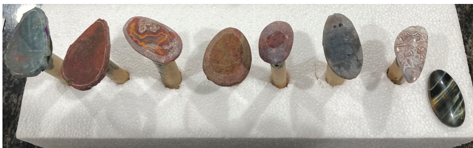
The progress of cabs from trimmed slab to finished cab
